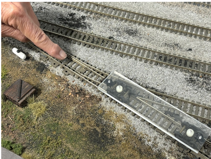
Figure 1 – Railroad inspection cars are used to assess whether switches or track are installed correctly to avoid derailments or to prevent the striking of objects along the right-of-way. The clear acrylic base allows you to see what is happening as wheels roll on tracks underneath the car. Cars like this are available from MicroMark, Walther's, or other vendors.
