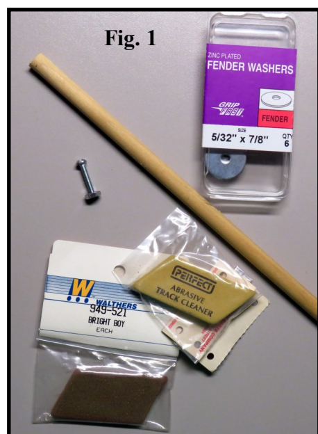
Figure 1 – The materials needed to create a cleaning rod for abrasive styles of track cleaners.
